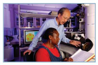
Joanita Jakana and Wah Chiu are with a JEM3000SFF electron cryomicroscope, a 300 kV electron microscope that can keep specimens at liquid helium temperature for cryo-electron microscopy experiments.
